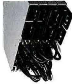
Figure 7. Cisco Catalyst 9300 Series StackPower
