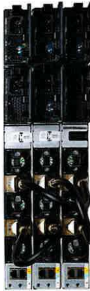
Figure 6. Cisco Catalyst 9300 Series fixed uplink models with optional stack kit
